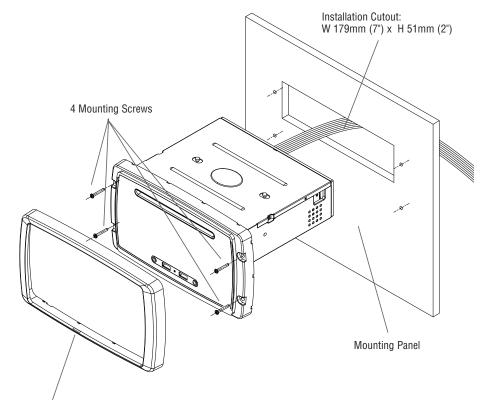
Trim Ring Notch Use small flathead screwdriver here to carefully remove trim ring.
